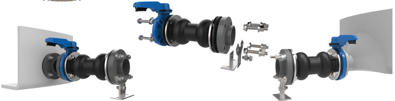
PVC/EPDM Valve, EPDM 2-Arch Expansion Joint with Galvanized Back-Up Rings, 304SS Adjustable-Height Support, PVC Mating Flange and (2) Galvanized Bolt Kits
